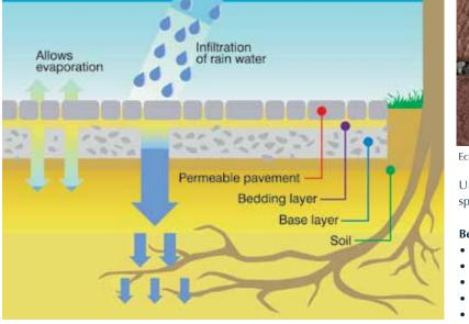
Illustration of the Unilock Permeable Pavement System
