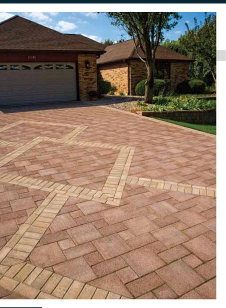
Series 3000<sup>®</sup>, a sophisticated paver with a high-performance surface, is made from a combination of granite and quartz particles. These brilliant speckles of color will remain 100% colorfast and will not fade or wear off. Series 3000<sup>®</sup> is perfect for residential or commercial driveways, walkways, patios and more and is available only from Unilock.
