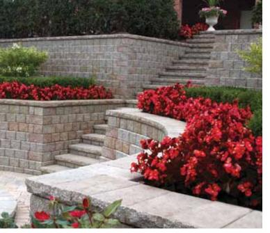
The built-in setback design of Pisa2® automatically forms the correct slope, ensuring a highly stable retaining wall. Utilizing the product's tapered components, you can form curved walls and steps.
